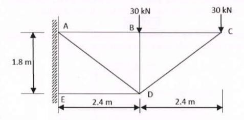
11 Analyze the members of a inclined truss loaded as shown in fig.
