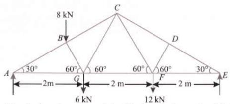
Determine the nature and magnitude of the forces in the members BC, GC and GF of the truss.
